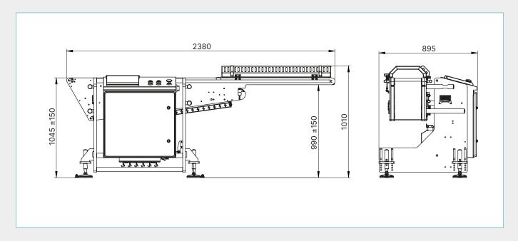
Specifications and photos are intended as a guide and can be changed by QUPAQ without notice. We make reservations for misprints and typing errors. The illustration and specifications are of the QUPAQ Shuttle Conveyor - 900. Item no. 90002657.
