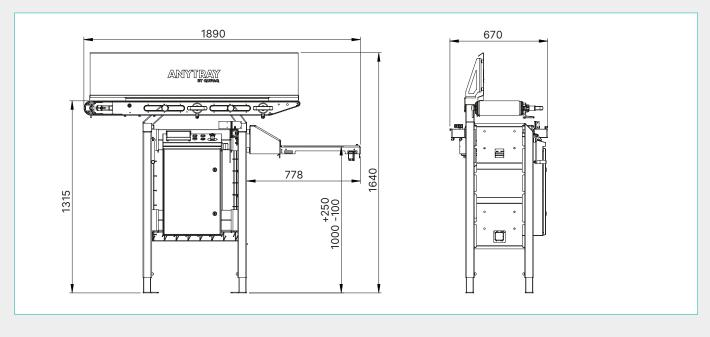
Specifications and photos are intended as a guide and can be changed by QUPAQ without notice. We make reservations for misprints and typing errors. The illustration and specifications are of the ANYTRAY Cleanline Buffer - 1500. Item no. 6010040314.
